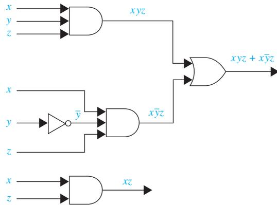
**FIGURE 1** Two circuits with the same output.
