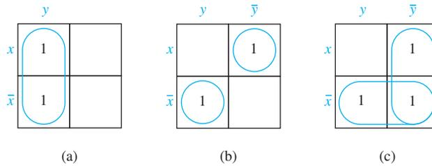
**FIGURE 4** Simplifying the sum-of-products expansions from Example 2.
