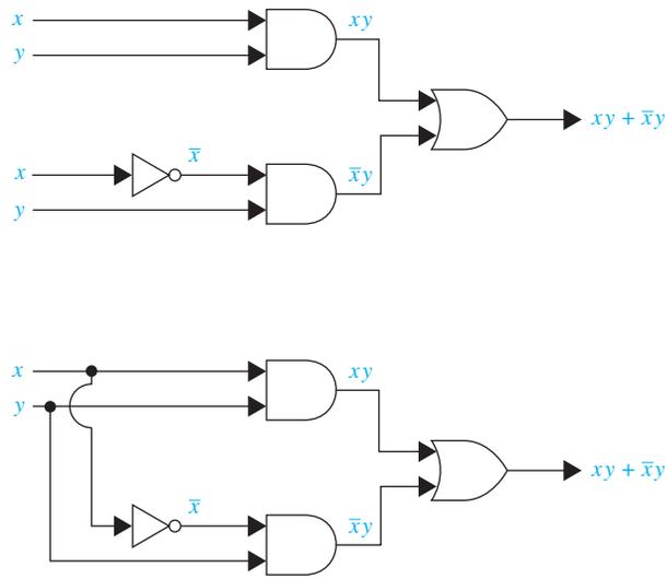
**FIGURE 3** Two ways to draw the same circuit.
