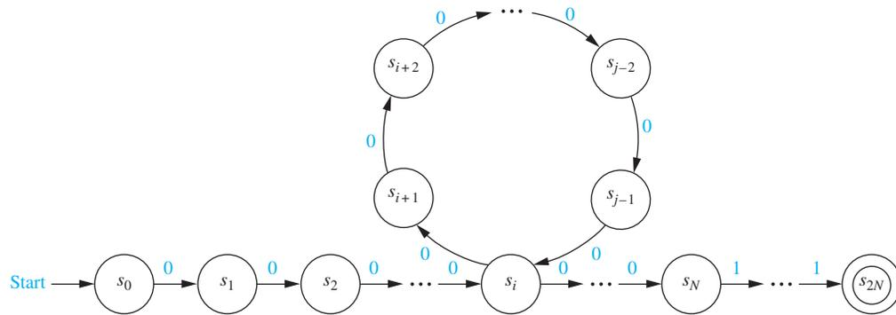
**FIGURE 6** The path produced by  $0^N 1^N$ .
